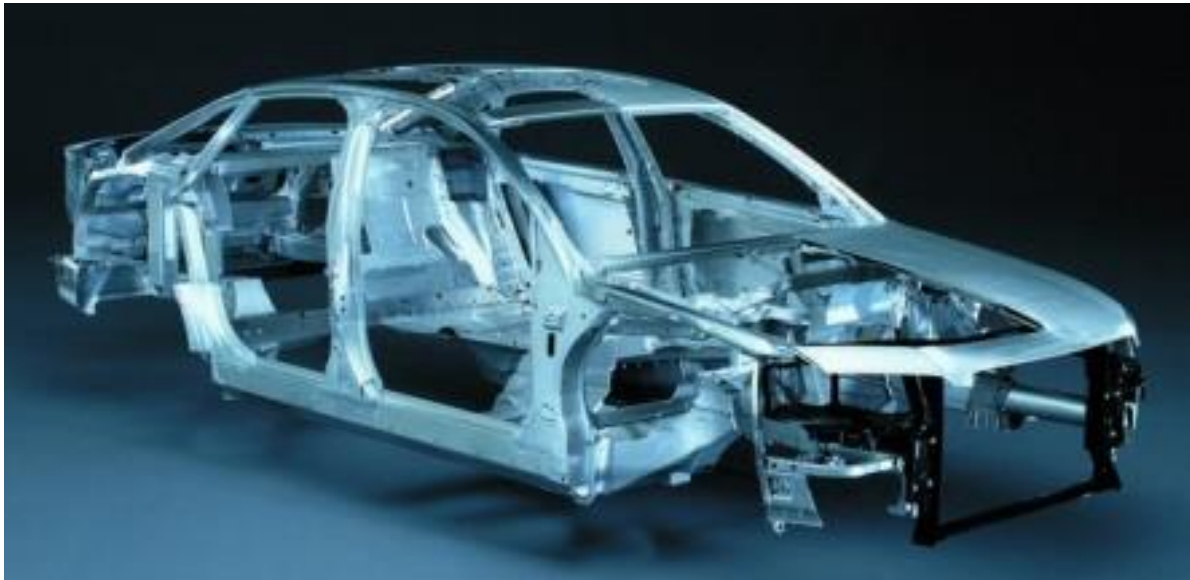
Audi A8 Aluminium Space Frame
